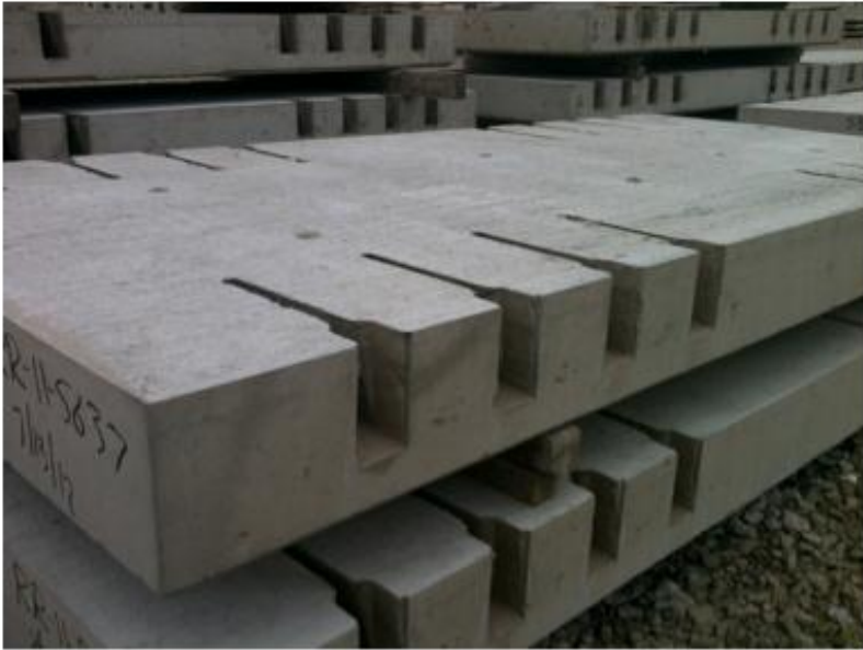
Utility Concrete in Morris, IL is supplying the precast slabs being used in the I-294 rehab project.
